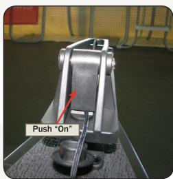
10. Secure the rope and anchor in place by pushing the Rope Lock to the "On" position.
