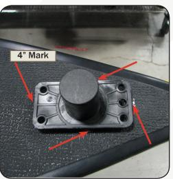
2. Locate the base attached to the Anchor Flush Mount(A). Pull and twist off to use as a jig. Align the mount upsidedown and forward of the 4" mark. Mark the three remaining sides.
