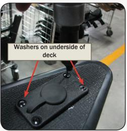
6. Insert the Rivets(C) and add Backup Deck Washers(D) to the underside of each rivet. Holding the washers in place, pop each rivet with a rivet gun.
