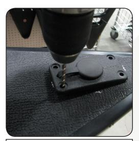
5. Use the 13/64" drill bit to drill out the four holes in the flush mount for the AA611D Rivets(C).
