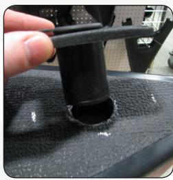
4. Insert the Anchor Lock Flush Mount(A) into the newly drilled hole.
