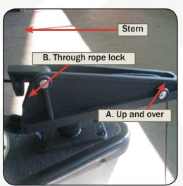
9. Feed the free end of the Rope(E) through the bottom of the Flush Mount(A), up and over the roller toward the back of the boat, then through the rope lock as shown.
